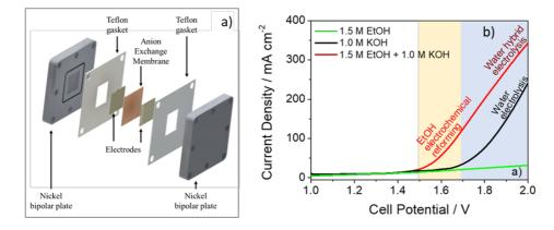
Figure 1. a) Exploded view of a complete electrolysis cell and b) current–potential curves for water and ethanol-water hybrid electrolysis.
