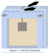
In order to obtain the metals' reduction, the MFC configuration was used for a period of 5 days, generating electrical current, reducing the  $Fe^{3+}$  to  $Fe^{2+}$  and recovering all the copper on the cathode surface. Then, the configuration is changed to MEC to get a total electrodeposition of metals.
